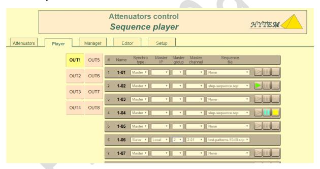
The player permits to launch sequences from the web server. In this case the attenuator number 2 has a sequence in memory named by the author "step-sequence.sqc" and the attenuator number 6 has his own sequence named "test-patterns-93dB.sqc" in memory.
