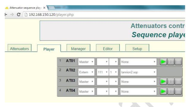
On this second subrack connection (120 here), the ATO2 WAY2 is choosen to be the slave of the subrack (111) (Extern) and the WAY1 (1). This slave way has it's own sequence
