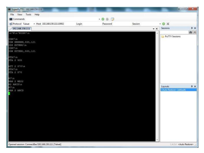
HOST: Input the IP address of the subrack then input the PORT number.
