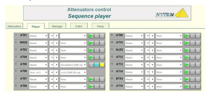
The player permits to launch sequences from the web server. In this case the attenuator number 6 has a sequence in memory named by the author "cyclic-93dB-20s.sqc" and the attenuator number 5 has his own sequence named "test-patterns-93dB.sqc" in memory.
