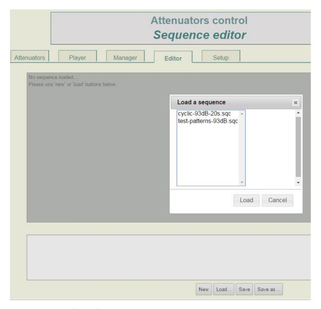
You can press "New" button to create a new sequence or Press "load" to read a sequence from the subrack SSD drive, choose the sequence you want to modify.
