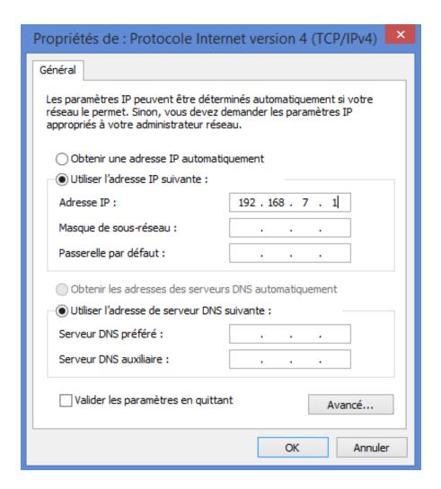
After setting the address and mask, click "OK" and back out of the dialogs. You have now set up the RNDIS network adapter!
