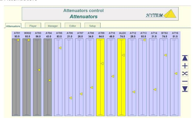
The first 4 attenuators are actually remotely connected by one or more users. They are greyed and you cannot move them. You can select attenuators you want to move, background become yellow, then you can change their values with your mouse, the "+" button, the "-" button, the Max or Min buttons or make a handover with the "cross" button.
