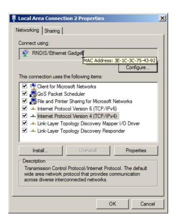
Double click the "Internet Protocol Version 4" setting line, and set the host address of the connection. In this example, I'm using 192.168.7.1 which is my host address, NOT the target address of the Hytem subrack.
