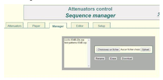
Sequence are uploaded/downloaded into or from the SSD drive with the computer you are using with the **Manager.**
